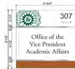
Primary ADA Room ID (MD) 5.0-ID/5.5 on a Common Backplate with Laminate Base Accent 5.0-ID Full Bleed Screen Top
