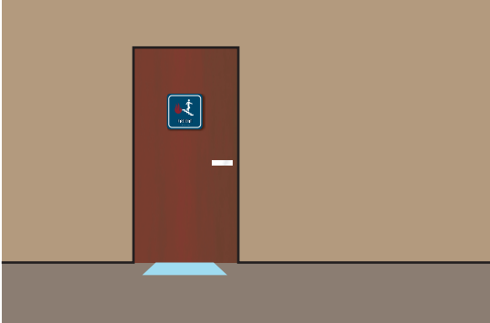
Located on Push Side of Door if Door Opens Inward and Does Not have a Hold-open Device
